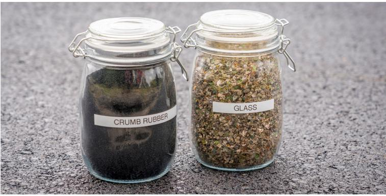
It is the first-time bitumen modified with waste tyre material – which included the equivalent of 40,000 beer bottles of recycled glass, as well as the end-of-life truck tyres – has been used in Tasmania.
