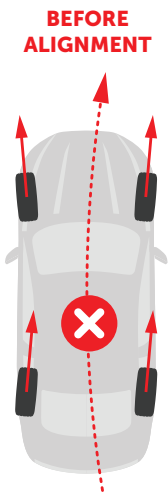
Pre-alignment angles out of specification
