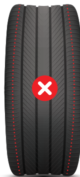
Excessive Shoulder Wear
