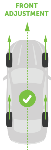
Steering wheel leveled – rear wheels measured and adjusted
