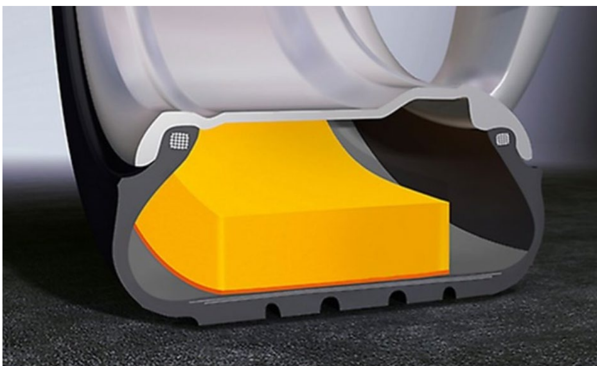
Figure 6: Passenger car tyre with a polyurethane noise reduction foam layer
